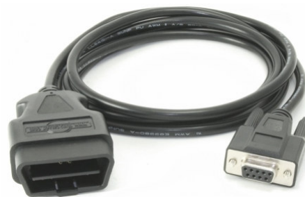
Fig. 7.2.2 OBD2 (On Board Diagnostics version 2) to serial interface
