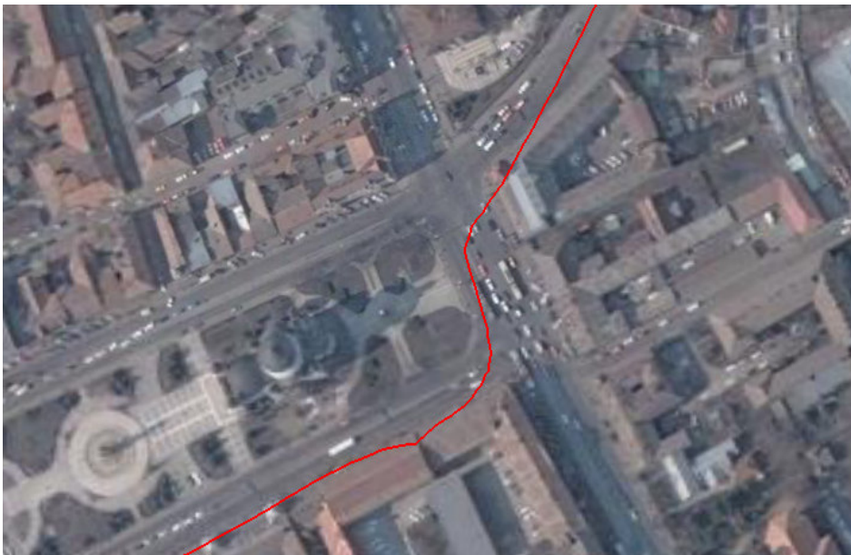
Fig. 2.3.1 GPS Data showing error, projected on calibrated satellite image
