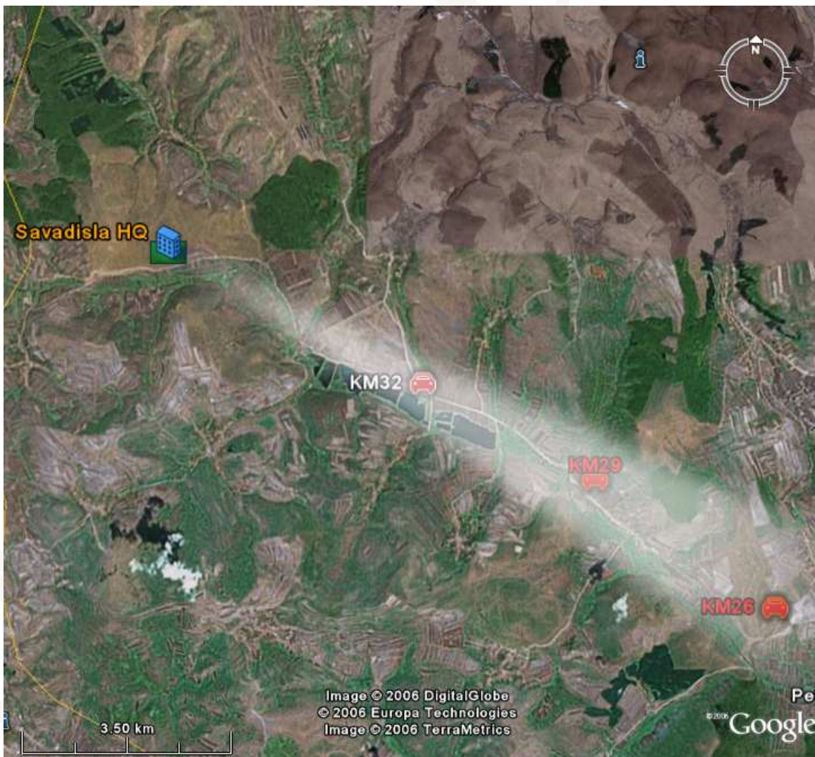
Map of the links with simulated 12.5 degree beamwidth.
